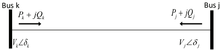
Figure 1 Busbar structure for formulation
