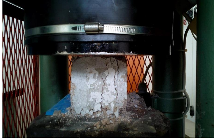
Figure 4. Execution of compressive strength test on concrete specimen
