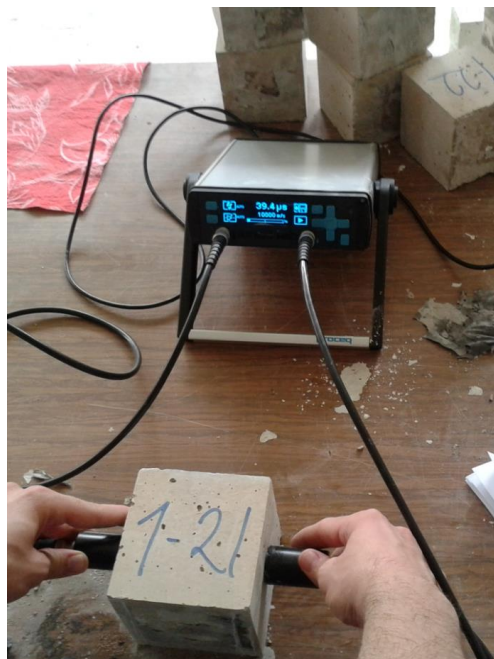
Figure 3. Ultrasonic pulse velocity test set up
