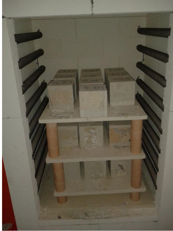
Figure 2. The oven used for the high temperature exposure and the specimens
